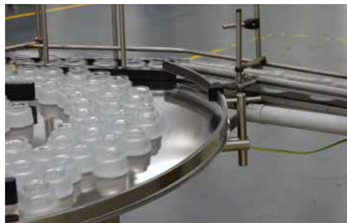
Closely packed: the glass crucibles undergo the vision inspection
